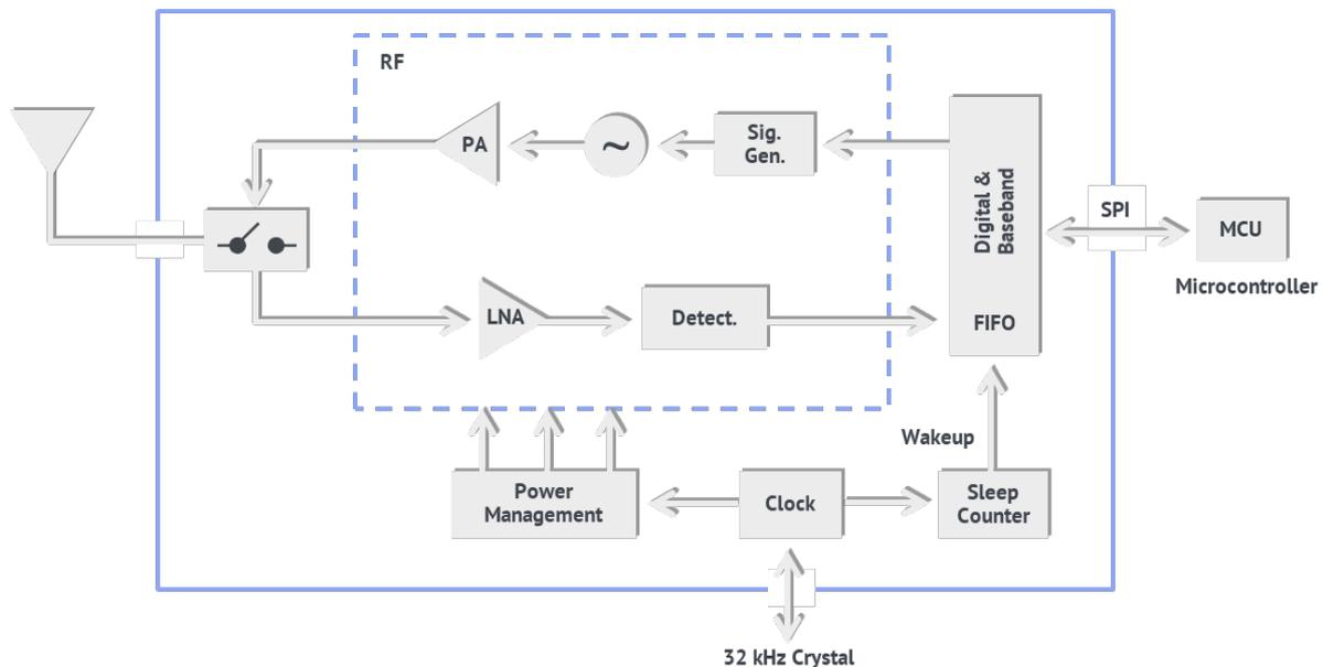
**Figure 9 – The SPARK Microsystems SR1000 series UWB transceiver functional block diagram. (source SPARK Microsystems)**
