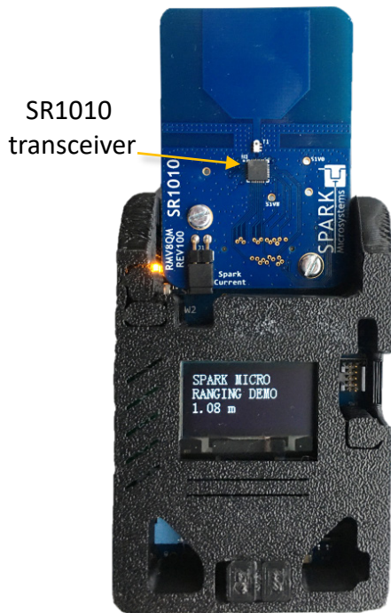
SPARK ranging evaluation kit with on-screen display*
