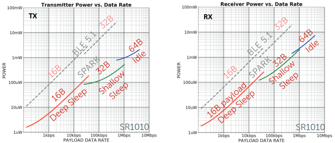
Figure 12: SR1010 TX (left) and RX (right) power consumption at 1.8V Supplies, compared to Bluetooth 5.1
